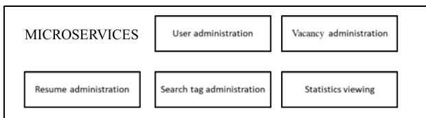
Fig. 2. Structural diagram of the microservice architecture of the administration panel
